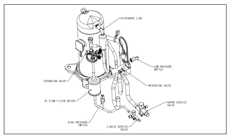
Figure 2. Typical Parts Arranegment - HRG15S1R
