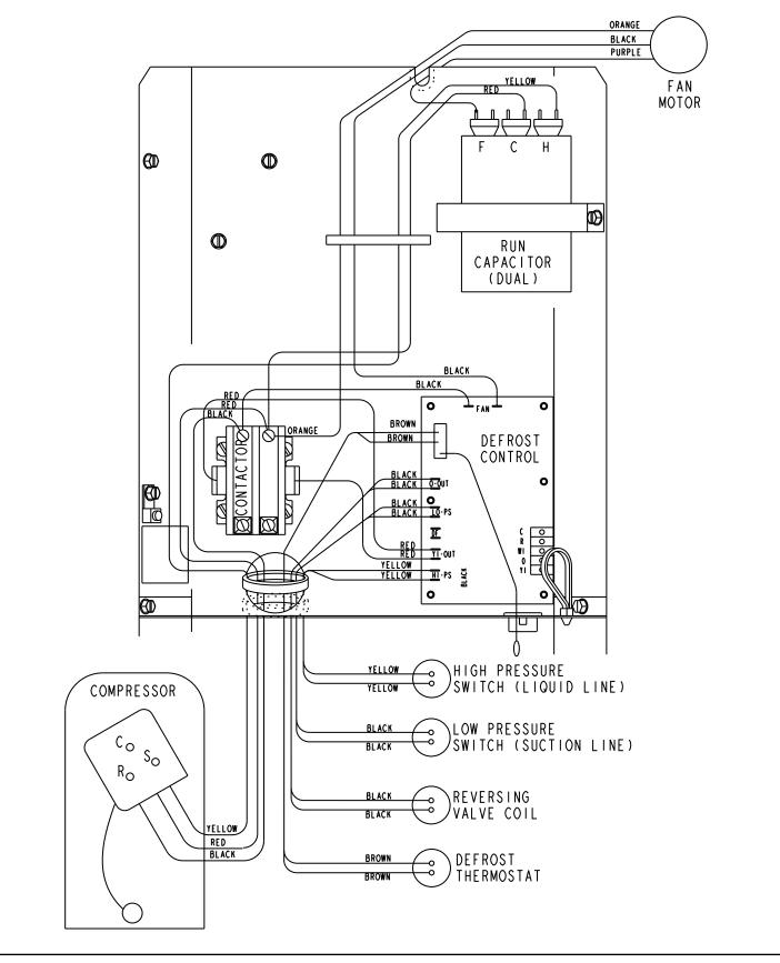
Figure 11. Typical Factory Wiring (-018 through -036 models)
