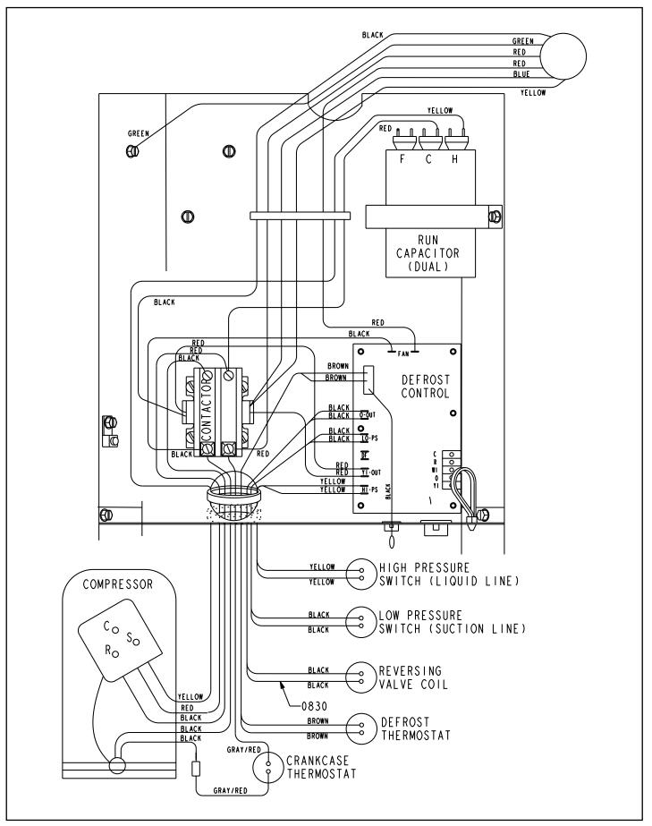
Figure 12. Typical Factory Wiring (-042 through -060 models)
