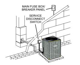
**NOTE** - Units are approved for use only with copper conductors. Ground unit at disconnect switch or connect to an earth ground.
