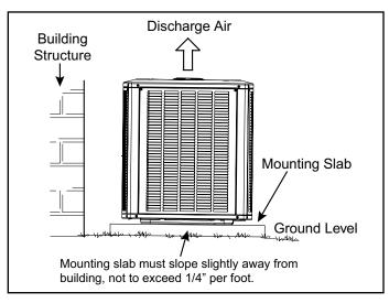
Figure 3. Slab Mounting
