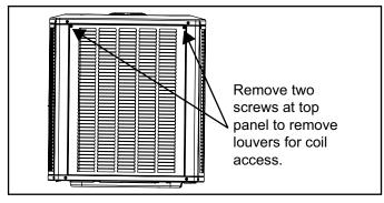
Figure 9. Removing Louvers
