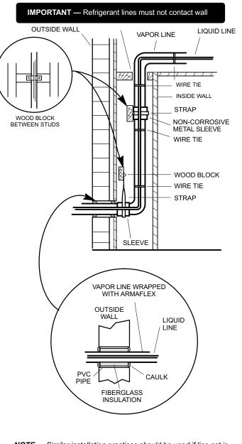
**NOTE** — Similar installation practices should be used if line set is to be installed on exterior of outside wall.
