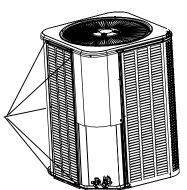
STEP 1 TO REMOVE PANEL, REMOVE MOUNTING SCREWS SECURING PANEL TO THE UNIT.
