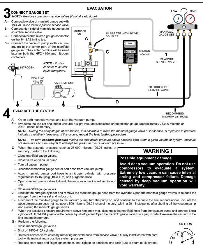
H - Open suction service valve first before liquid valve to release the unit charge into the system. Replace valve caps and tighten (8 ft. lb.). Caps are the primary seal.
